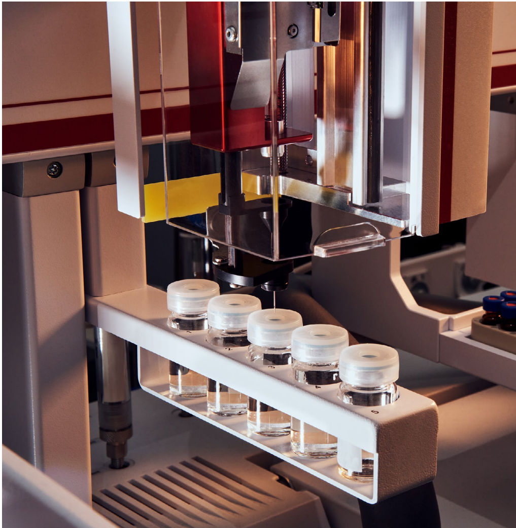
We evaluate materials for substances restricted in our Regulated Substances Specification — including VOCs — using equipment like this gas chromatography/mass spectrometry (GC/MS) system.
