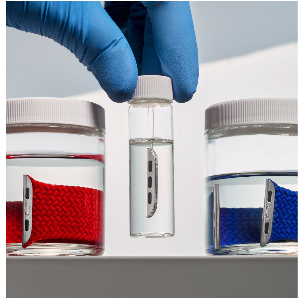
We test all our products, and place special attention on materials that come into prolonged skin contact. In this nickel leach test, we place Apple Watch bands in jars of artificial sweat to ensure the nickel, a potential allergen, stays where it belongs — in the product.
